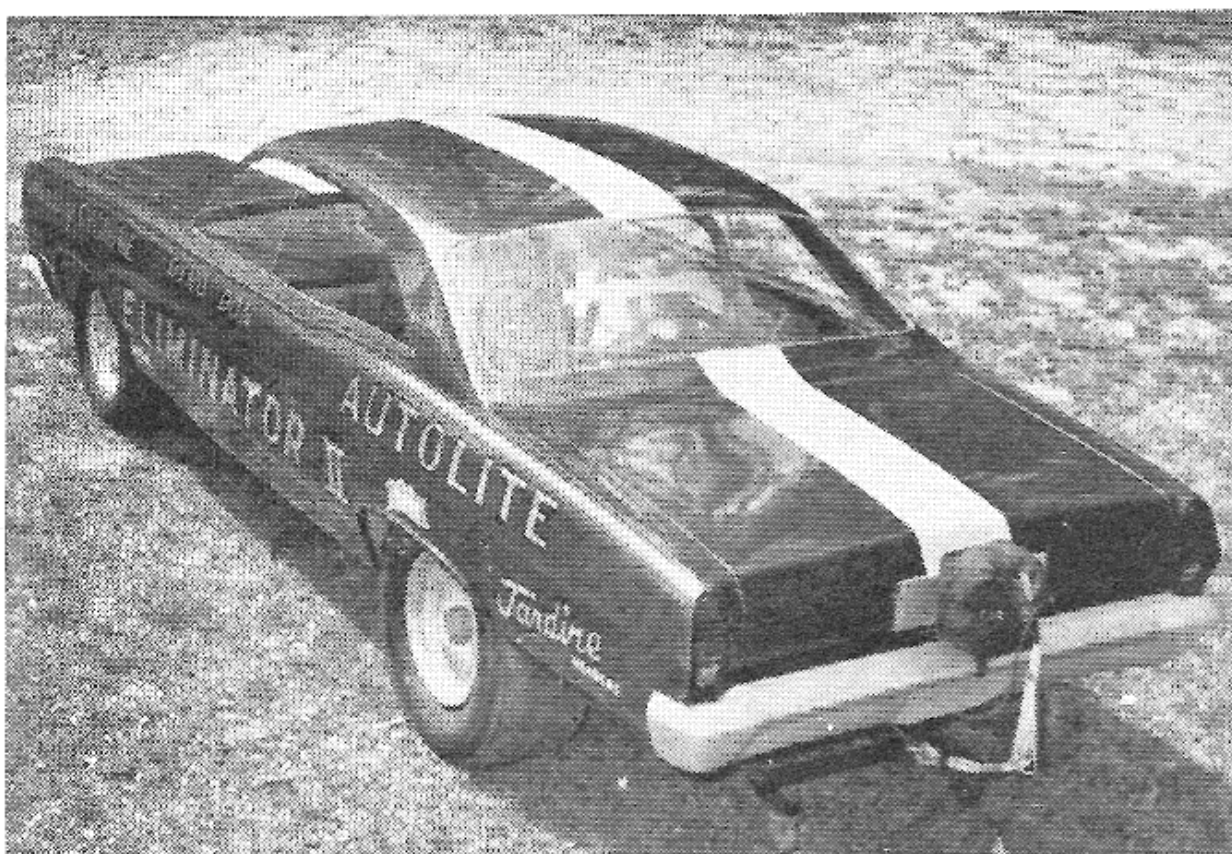
ABOVE — To comply with a current NHRA rule, this "emergency only" escape hatch was built into car. Pop rivets hold it in place, but pressure removes it quickly.
