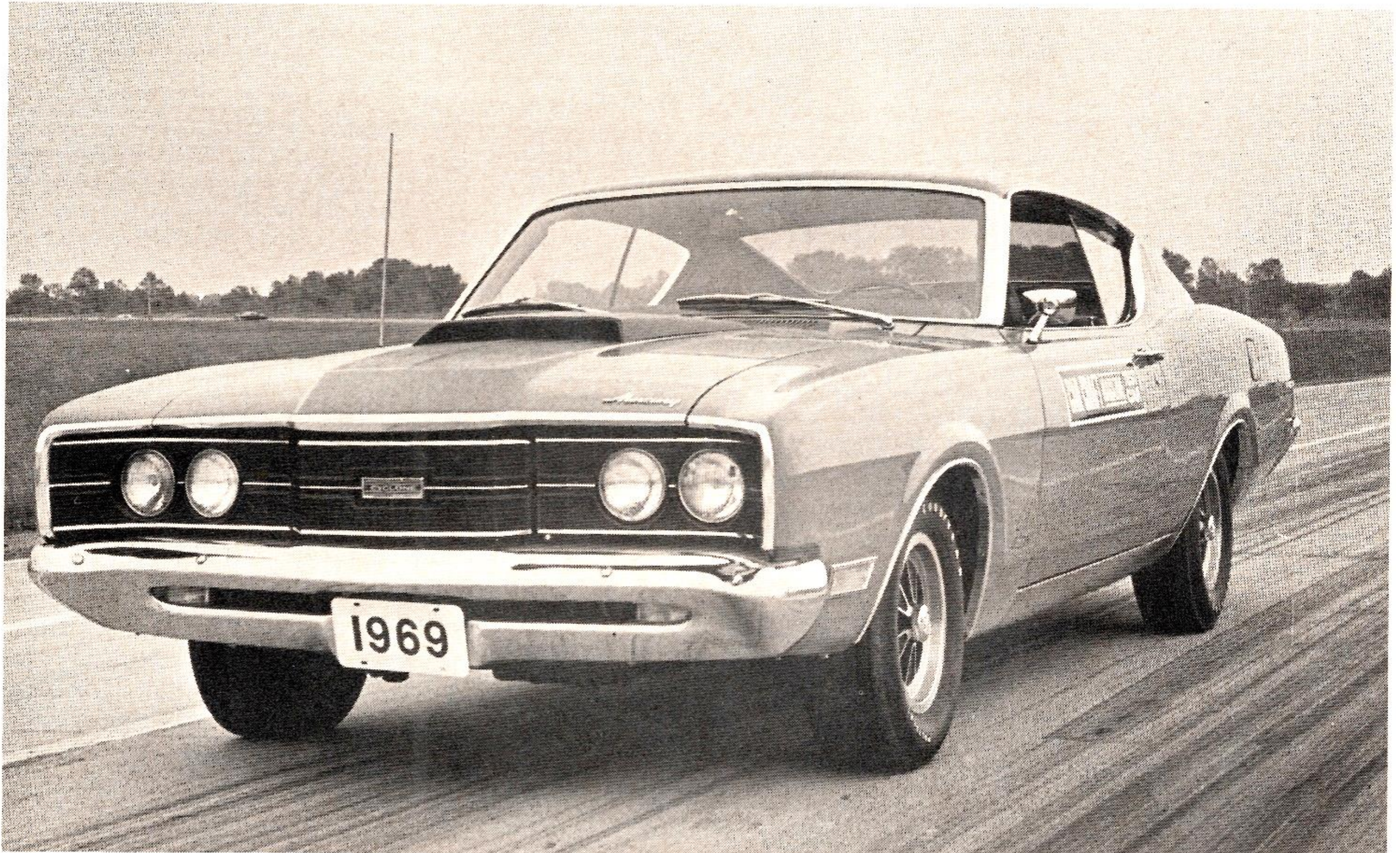
Our test Cyclone had the CJ 428 mill, automatic, 3.90 gears, power steering, and power disc/drum brakes, had no trouble cutting 14.0's and 100+ mph. Goodyear Polyglas tires gave plenty of traction. All hood scoops are functional, as only Ram Airs have 'em.
